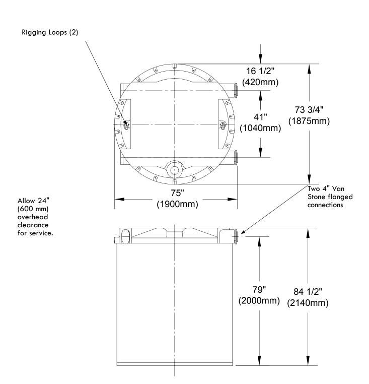
**NOTE:** Tolerance for all dimensions is  $\pm 1/2$ " (12.5 mm)
